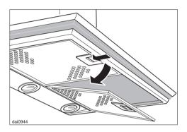
To remove the grease filters press the locking clips in towards the middle of the filter. Support grease filter so that it does not fall on to the cooktop. Clean the filters
